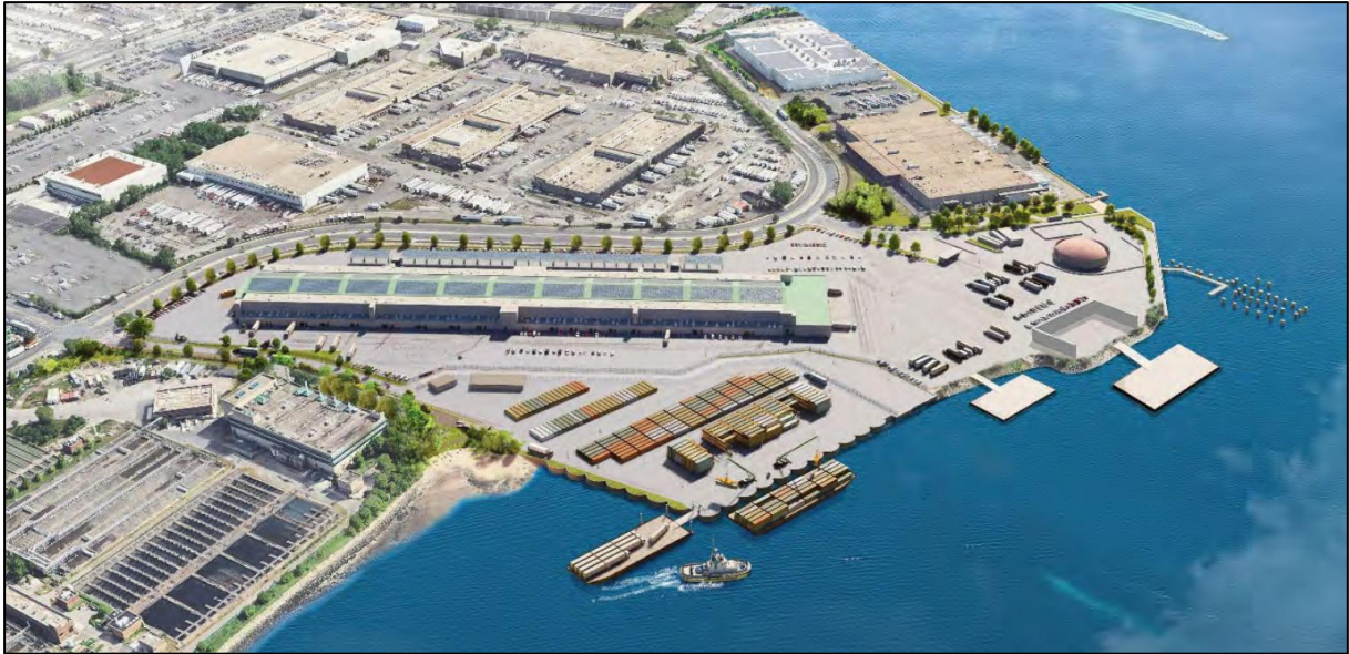
Fig. 9: Artist impression of the planned new facility at Hunts Point (the two cranes shown on the image handling containers at the quayside from a conventional barge are much too small: to handle containers massive and expensive mobile harbor cranes would be needed, but can be saved when deploying Port Feeder Barges), source: NYC DOT & NYC EDC
