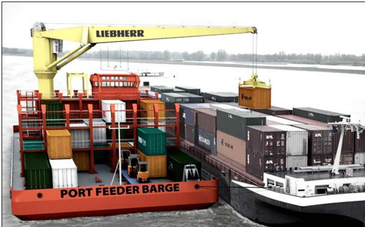
Fig. 11: The Port Feeder Barge is serving an (European) inland barge midstream (computer rendering)
